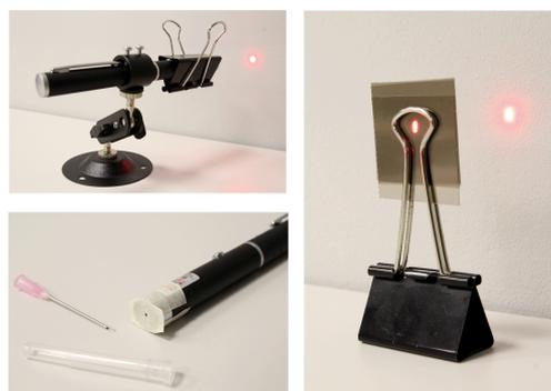
Figure 19: Laser is kept switched on using large clip. To reduce beam size use sticky tape and a needle. Darkening film in a holder (large clip) to reduce laser intensity.
